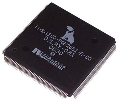
Figure 1. The fido microcontroller packaged in a 208 PQFP
